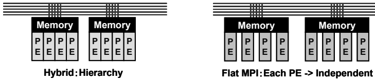
Fig. 1. Parallel programming models on SMP cluster architecture [1,2]
